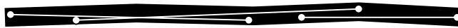
Figure 10.21: Three line detectors for what should be seen as a single line segment
