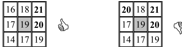
Figure 10.10: Example of endoskeleton pixel on the left, and counter-example on the right
